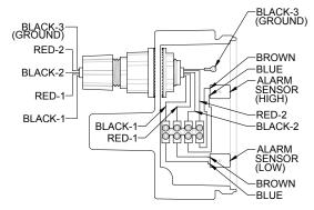
**DUAL ALARM WIRING DIAGRAM**
