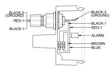
SINGLE ALARM WIRING DIAGRAM
