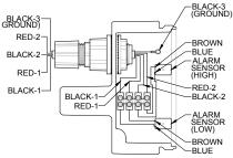
**DUAL ALARM WIRING DIAGRAM**
