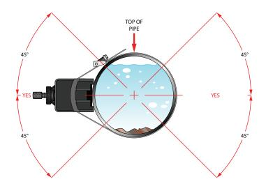
Figure 1: Transducer positioning
