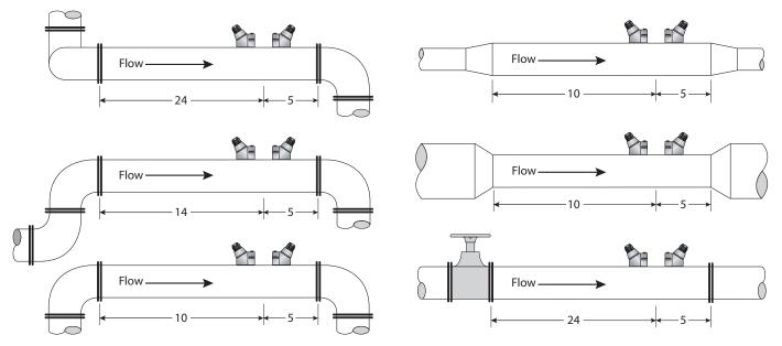
Figure 2: Piping configuration and transducer positioning
