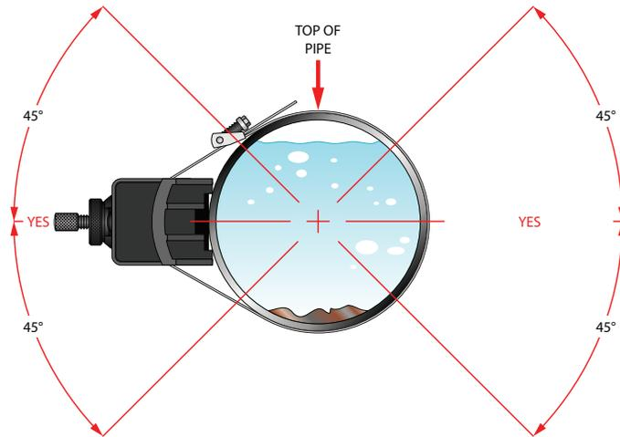
Figure 1: Transducer positioning
