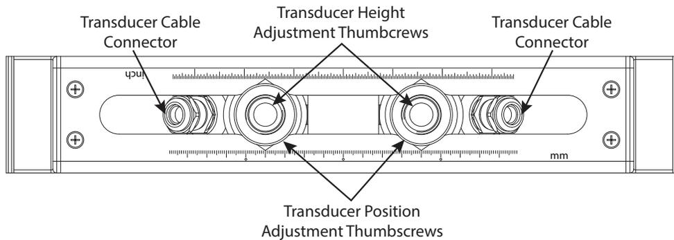
Figure 5: Easy rail top view
