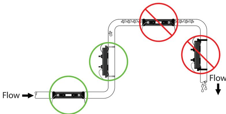
Figure 3: Transducer orientation
