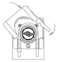
3) Close the compression block and fasten the trigger.
