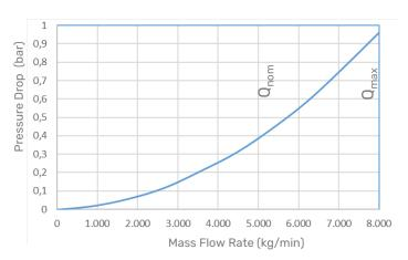
0 – 8000 kg/min water, sensor with P1 pressure rating. Higher viscosities create higher pressure drop
