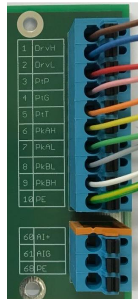
Figure 2: RHE21 Wiring with RHM Connection Type TM
