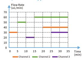
Parameters programming through dedicated PC software can achieve complex flow profiles for four drive units
