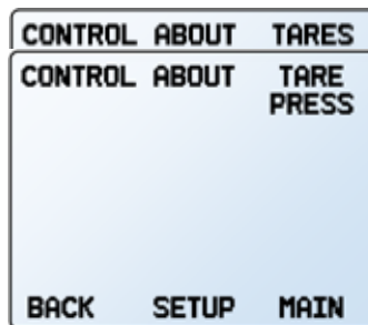
Flow devices have a TARES option while pressure devices have a TARE PRESS option on the main menu.
