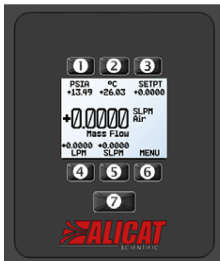
Live screen of a mass flow controller measuring the mass flow of air.
