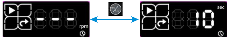
Display the Speed in the Prime Status (Timer mode)
