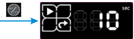
Display the Accumulated Run Time in the Prime status (Continuous mode)
